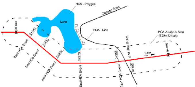
Example where the user has specified an Analysis area using an event based Analysis area (i.e. Thermal Radiation)
